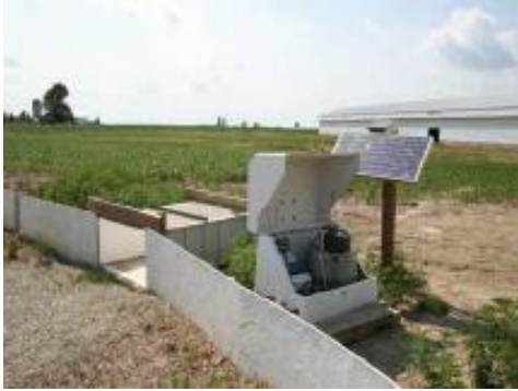
Figure 1: Edge-of-field surface runoff site with a 2.5 foot H-flume.
