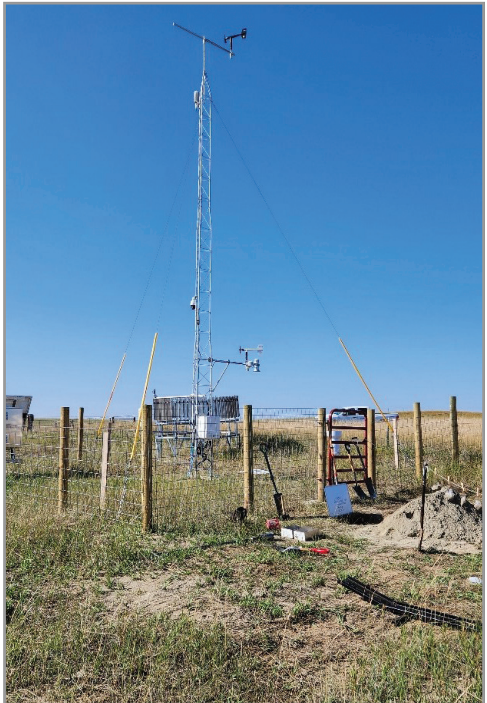
Figure 24.—Installation of an Upper Missouri River Basin Monitoring Network station to monitor snowpack and soil moisture.
