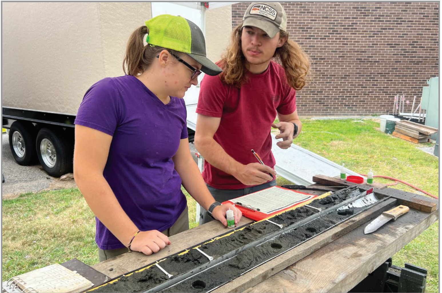
Figure 36.—Soil and Plant Science Division soil scientists describe a subaqueous soil core collected as part of the coastal zone soil survey of Long Island Sound.
