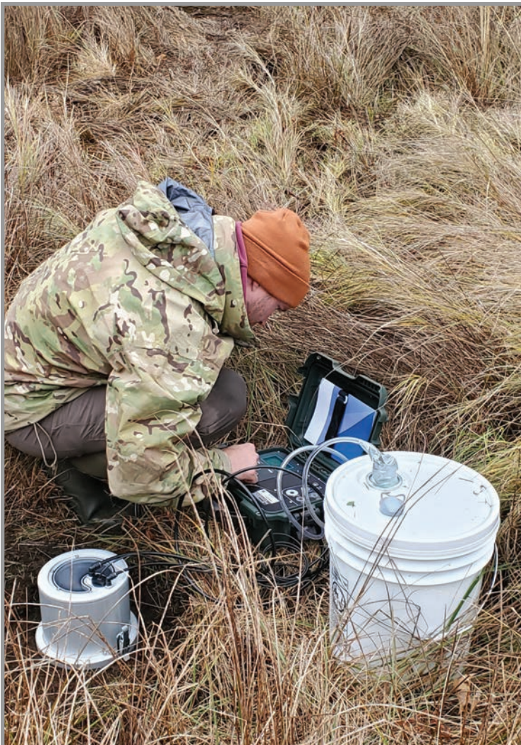
Figure 8.—A soil scientist in a grassy area sets up a Saturo unit to measure hydraulic conductivity.
