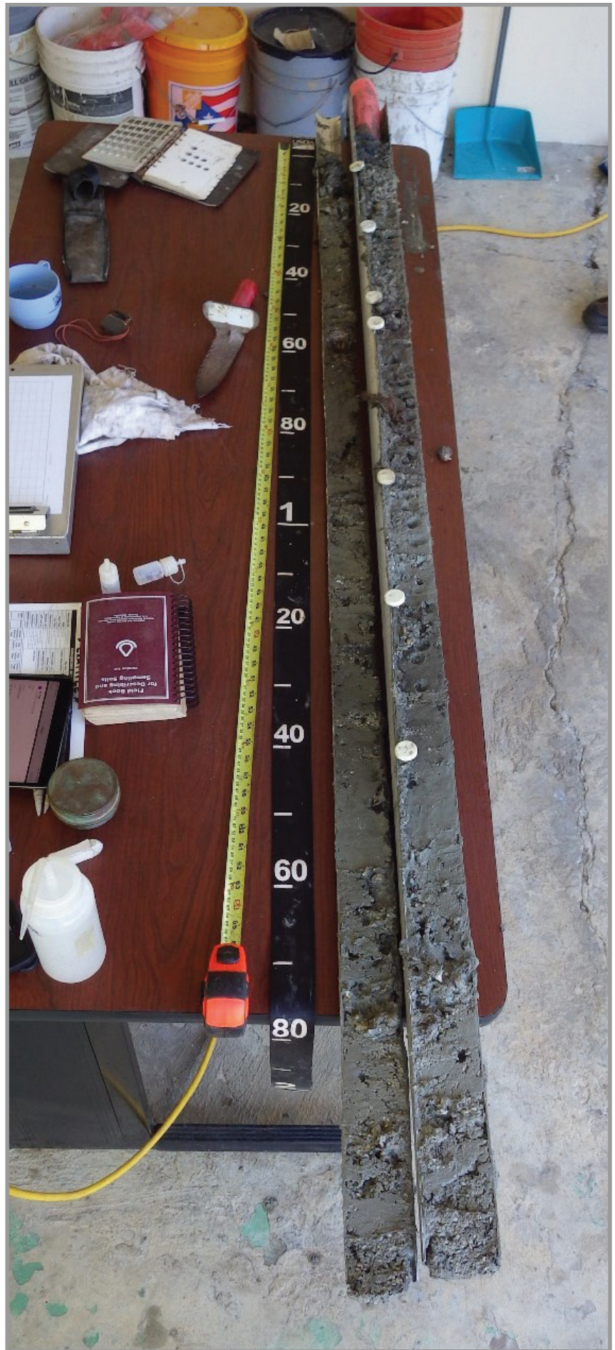
Figure 19.—An open subaqueous soil core from the coastal zone soil survey of Jobos Bay.
