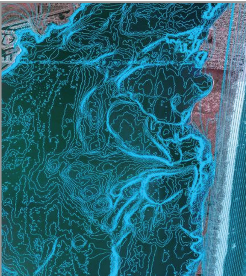
Figure 11.—Contours created by topobathymetric light detection and ranging technology are used for mapping subaqueous and coastal soils.
