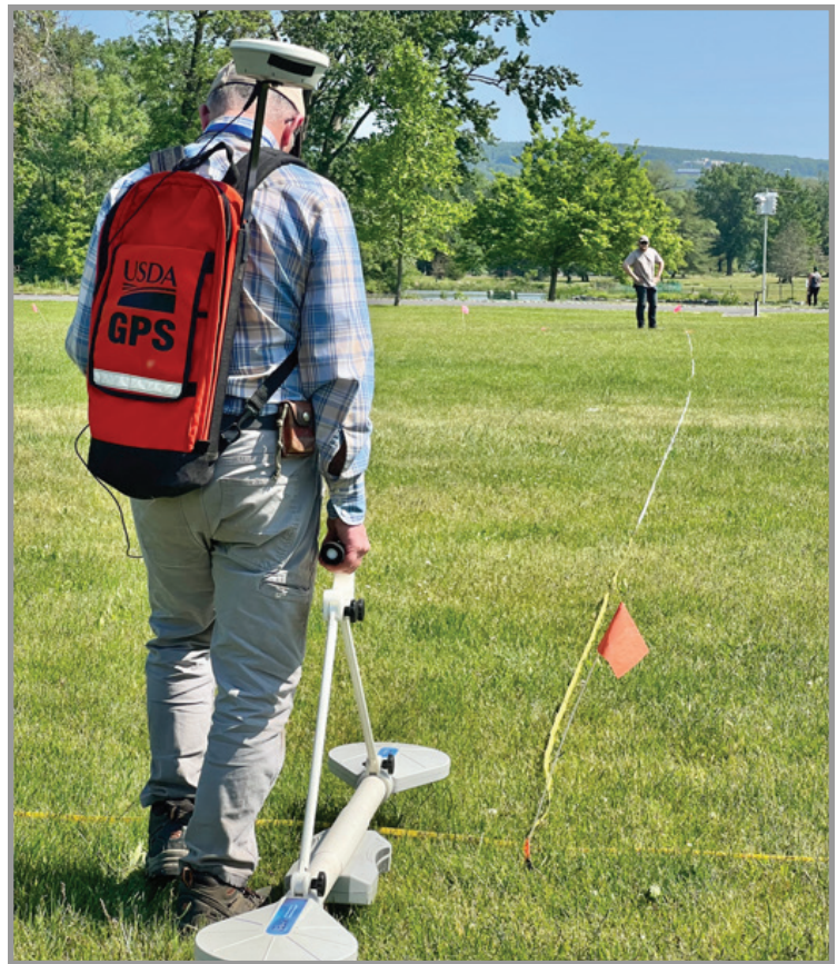
Figure 39.—Soil and Plant Science Division soil scientists use electromagnetic induction equipment to document the thickness of dredge spoil at the southern margin of Lake Cayuga in a filled marshland.
