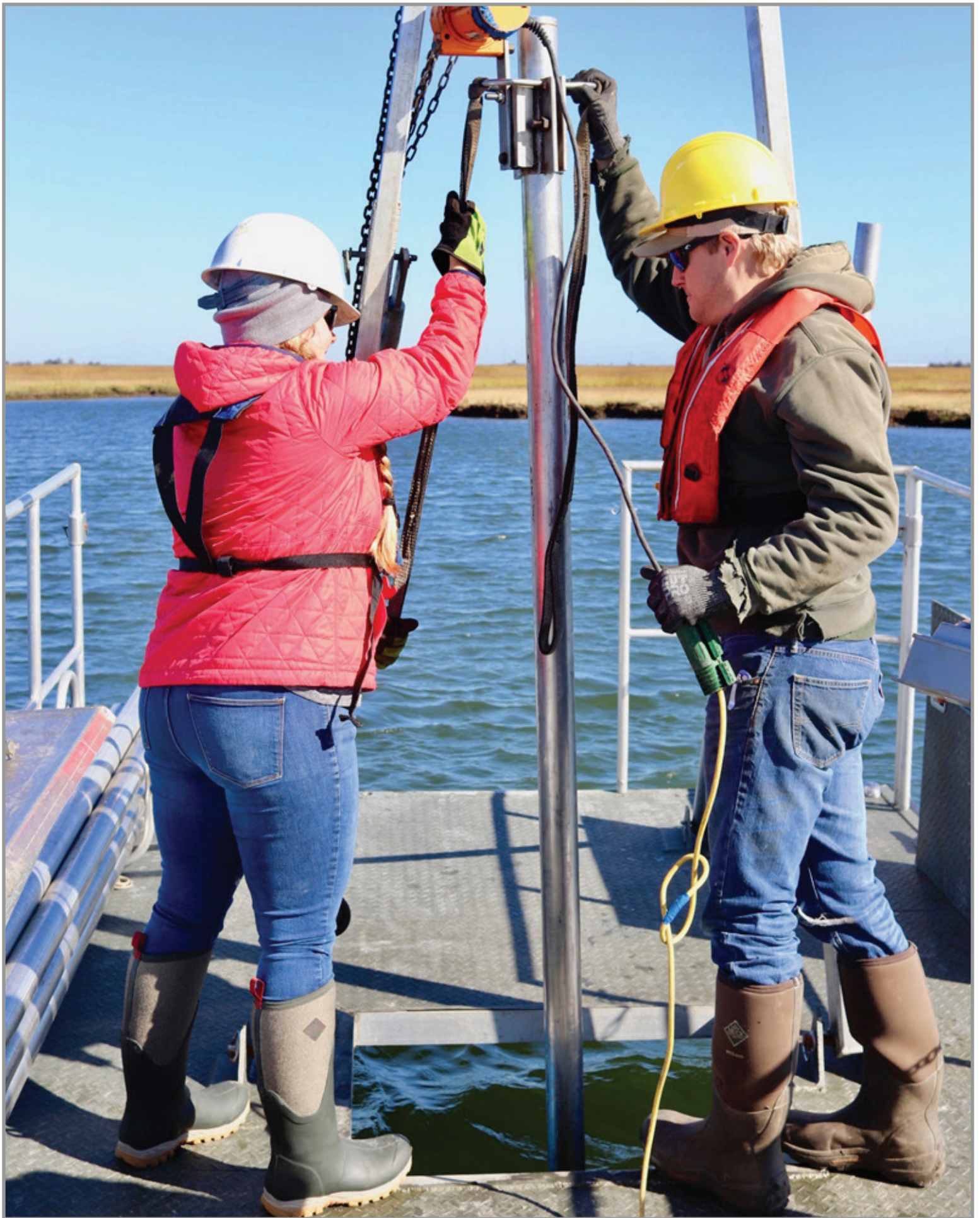
Figure 21.—Soil and Plant Science Division soil scientists collect a subaqueous soil core.
