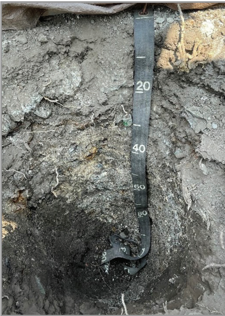
Figure 41.—A soil formed in coal ash (photo tape depths in centimeters) in Ithaca, New York, capped with clean fill materials.
