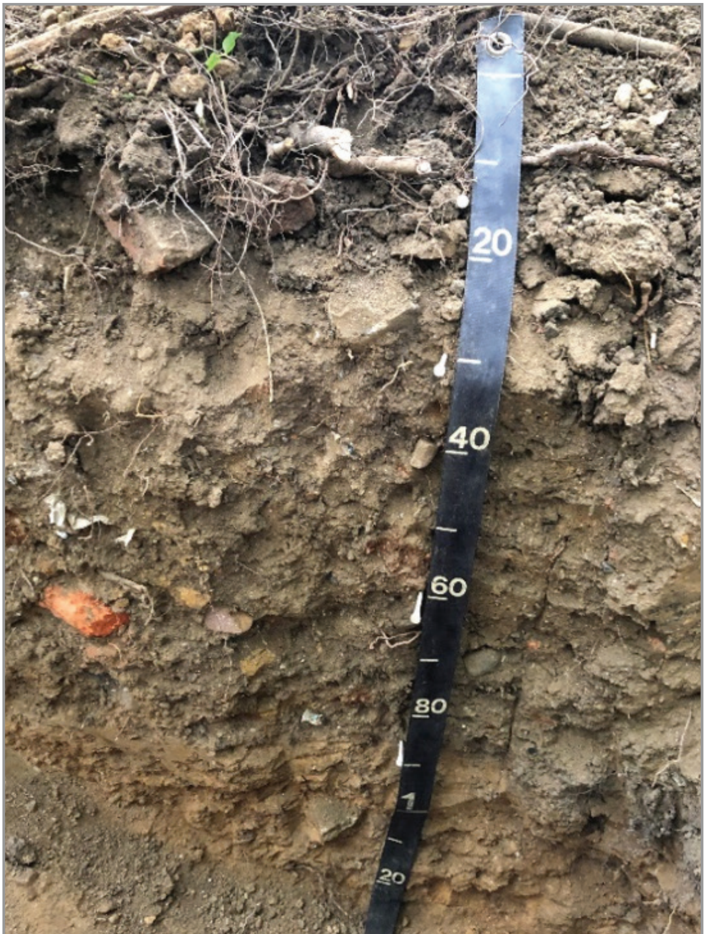
Figure 46.—A Folcroft soil profile, a new soil series formed in human-transported materials with a high content of human artifacts and rock fragments on raised human-created landforms.
