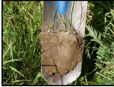
Figure 16: Using a sharpshooter to extract a slice of soil
