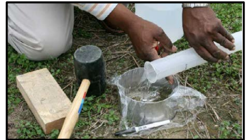
Figure 7: Preparing soil infiltration test
