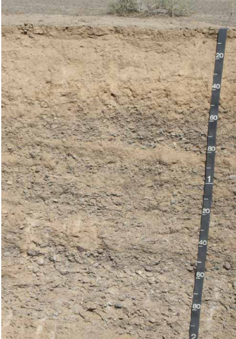
Profile of a Cambid (specifically a Haplocambid) in the United Arab Emirates. The cambic horizon extends from a depth of 10 cm to about 50 cm. Scale is in cm. (Photo courtesy of Dr. Craig Ditzler)
