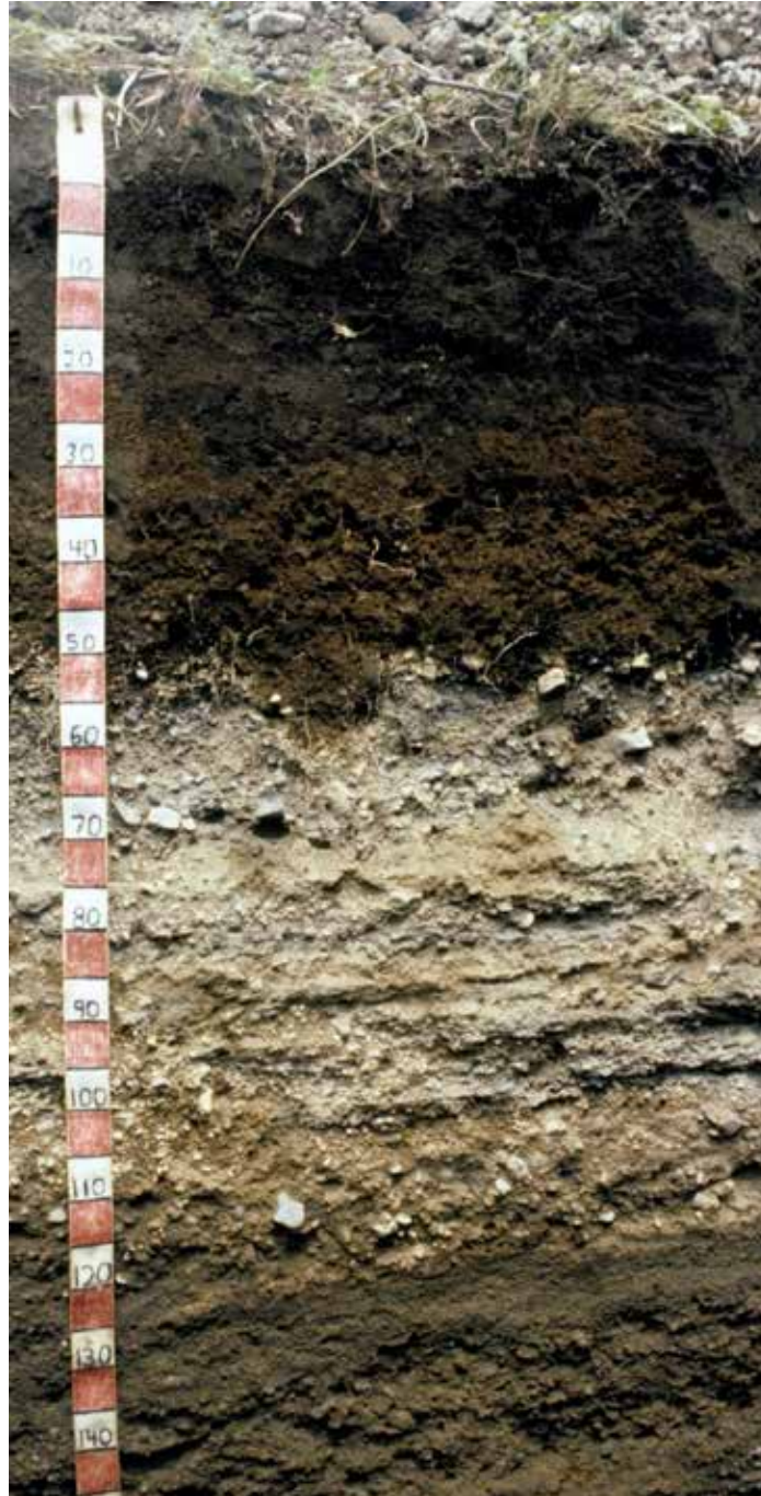
Profile of a well drained, gravelly Humustept in the Philippines. The soil formed in stratified layers of material, including volcanic ash. It has a dark, humus-rich umbric epipedon about 28 cm thick. Below this epipedon is a cambic horizon that extends to a depth of about 55 cm. Scale is in cm.
