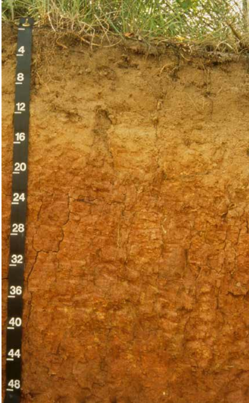
Profile of a Udult (specifically a Kandiudult) in North Carolina. This soil has an ochric epipedon about 12 inches thick underlain by a reddish yellow kandic horizon that extends below the base of the photo. Scale is in inches.
