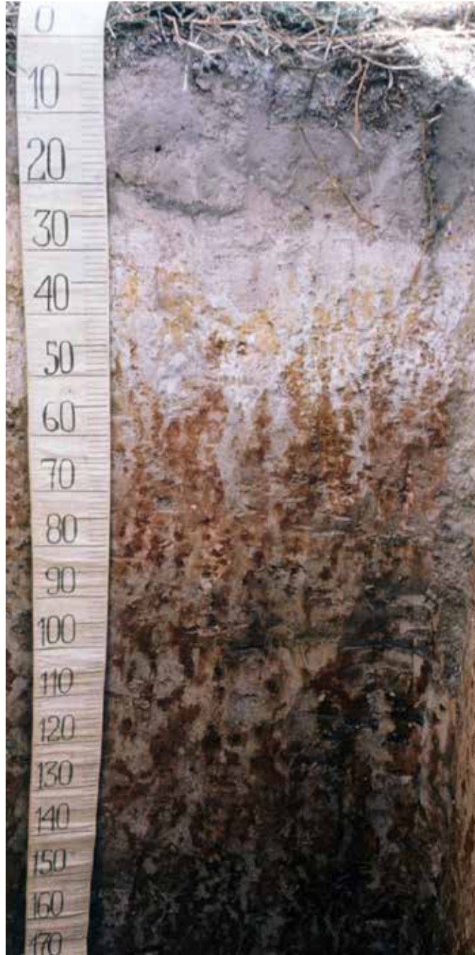
Profile of an Aquult (specifically a Plinthaquult) in Venezuela. Some of the red bodies in the subsoil are plinthite. Scale is in cm.
