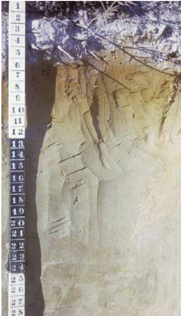
Profile of an Orthod (specifically a Haplorthod). The albic horizon (white) extends from a depth of about 1 to 5 inches and is underlain by a reddish spodic horizon that extends to a depth of about 11 inches. Scale is in inches.
