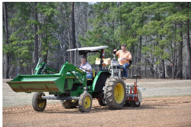
Planting wildflower mixes into a clean, prepared seedbed using a Hege 1000 research plot planter
