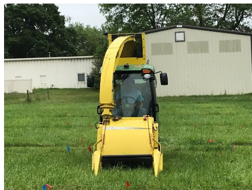
Figure 1: A RCI plot forage harvester is used to clip and weigh a plot of 'Max Q' tall fescue.
