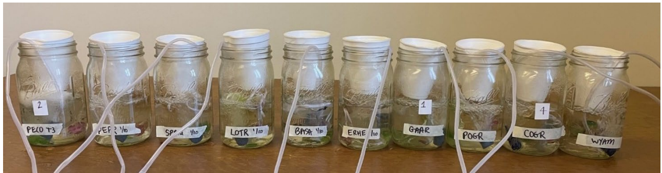
Figure 1. Seeds in drawstring bags, in mason jars with distilled water, connected to an air pump adding oxygen to the water.
