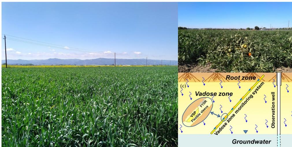
On the left: field in Spring 2020. Triticale was seeded in November 2019 as a winter cover crop, after processing tomato harvest. On the right: deep vadose-zone monitoring system to be installed in March 2020. This system will measure soil water content and will allow for soil pore water sampling from the root zone and up to the groundwater table. Nitrate concentrations will be measured all year round in two profiles.
